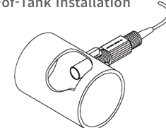
View 2 Pipe-line Installation with Reducer
