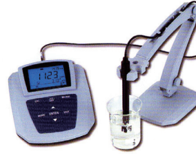
MP513 Lab. Conductivity Meter 측정 Parameters : Cond, resistivity, TDS, salinity 및 temperature
